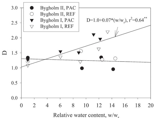
**Fig. 5. Relationship between the rupture energy–aggregate size scaling factor ( $D$ ) and the relative water content ( $w/w_0$ ) for the Bygholm soils. The lines are best-fit linear regressions; the relationship for the Bygholm II soil was not significant. PAC = compacted, and REF = reference treatment.**
