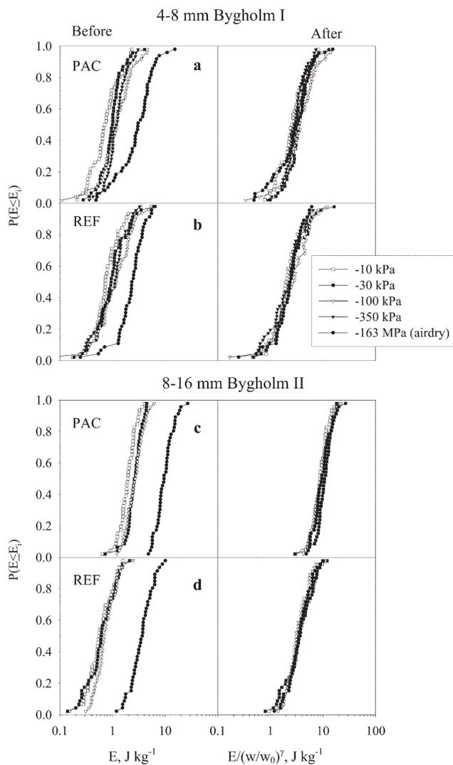
**Fig. 3. Cumulative density functions for the cumulative probability density function  $P(E \leq E_p)$  vs. specific rupture energy  $E$  before and after normalization of  $E$  to the air-dry state  $[E/(w/w_0)^\gamma]$  for (a) and (b) 4- to 8-mm Bygholm I aggregates, and (c) and (d) 8- to 16-mm Bygholm II aggregates. PAC = compacted treatment, and REF = reference treatment.**
