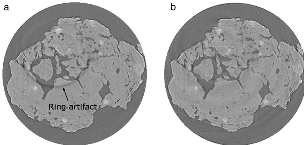
Fig. 1. Reconstructed slice before (a) and after (b) ring artifact correction.
