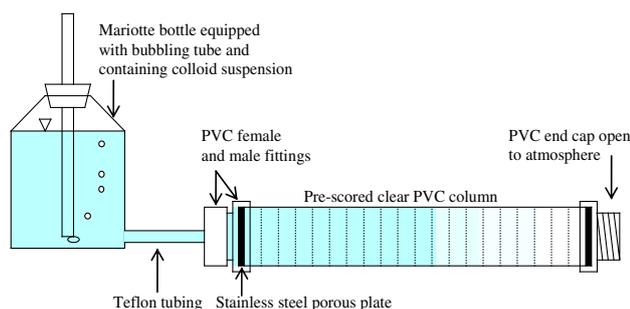
**Fig. 1 – Schematic diagram of the horizontal column system.**
